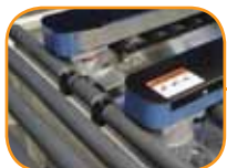
Twin ½ HP gear motors to process up to 85 lb cases
