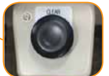
"Clear" button for jams & replacing bottom tape roll
