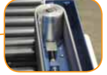
Self-tensioning & self-tracking drive belts simplify belt replacement
