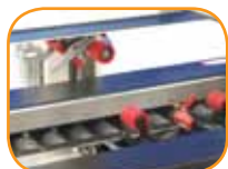
Offset 3" wide tape heads process cases as low as 5"
