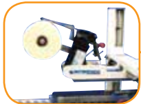
Tip up top tape head simplifies roll replacement
